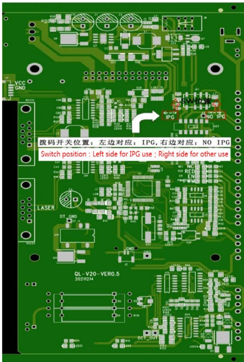
Figure 2.13 Schematic diagram of the dial code switch
