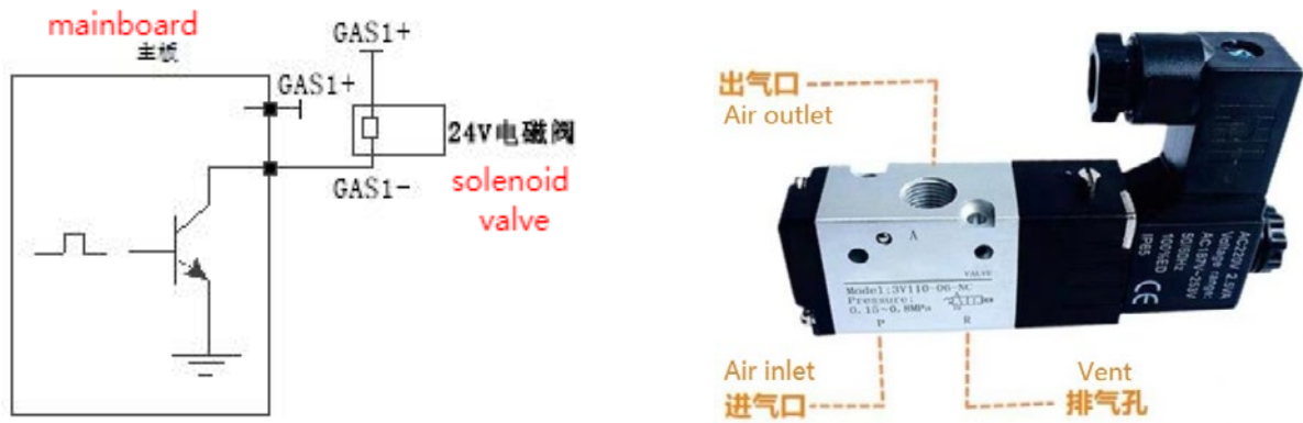
Figure 2.121 Schematic diagram of the gas control interface
