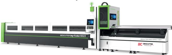
Our **HYTUBE** is designed for long-sized tube/section bar automatic laser cutting.
